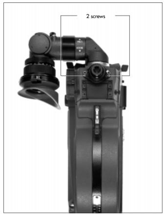
• Place the video optic back into the mount and close the two screws  $\triangleright$  **photo**.
