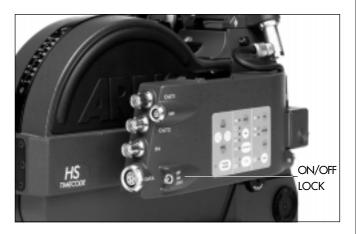
The OFF position switches the IVS off without affecting the film camera. ON activates the IVS, and LOCK disables the keyboard to prevent unintentional handling
