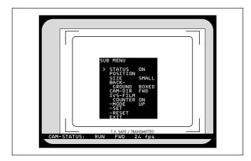
Like all man-readable information, the data is inserted as a window on the monitor image. The window can be switched on and off independently. Background, position and character format can be altered without affecting the settings of other windows.
