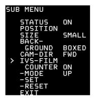
The sub menu line IVS-FILM COUNTER switches the IVS film counter on and off.
